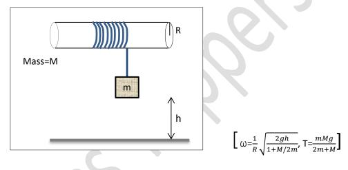
14. A carpet of mass M of inextensible material is rolled along its length in the form of a cylinder of radius R and is kept on a rough floor. The carpet starts unrolling without sliding on the floor when a negligible small push is given to it. Calculate the horizontal velocity of the axis of the cylindrical part of the carpet when its radius
